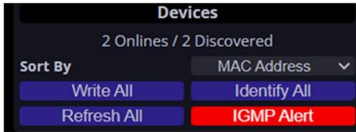
As IGMP snooping acts on multicast traffic, any action on a port **IGMP Mode** function or Group IGMP snooping enable/disable will activate the blinking IGMP alert in the Devices section.
