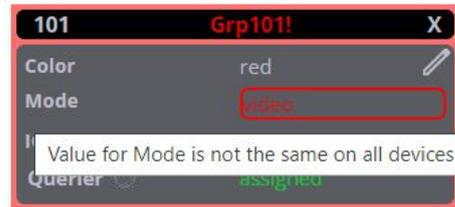
Red alert in Group means that Mode or IGMP settings are not the same in all devices for this group, or No IGMP Querier is assigned. This will cause Multicast traffic interruption.
