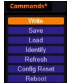
NB: When the device is **Discovered** but "**Offline**" due to IP mismatch or conflict, **Identify** is possible (except for I-series)
